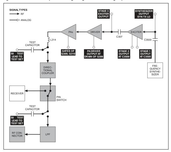
Task 26 — Output of Frequency Synthesizer The first point to check in the initial RF signal path is the output SYN TX LO from the frequency synthesizer. This signal is input to the exciter at C300.
