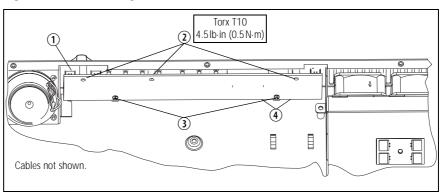
Figure 7.2 Removing the UI board
