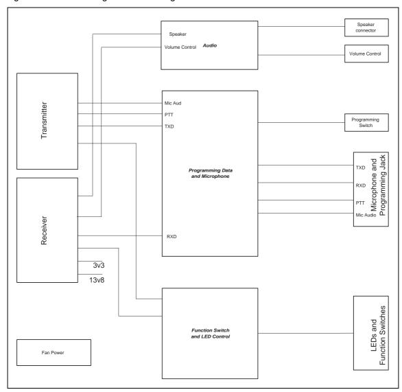
Figure 3.6 UI board high-level block diagram
