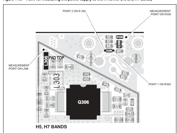
Figure 14.5 Point for measuring the power supply to the PA driver (H5 and H7 bands)
