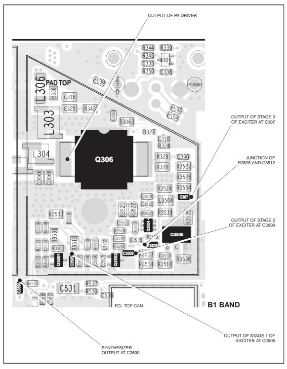
OUTPUT OF PA DRIVER R344 R339 R346 4308 C335 R350 C336 6100 **PAD TOP** R343 R324 31 C310 OUTPUT OF STAGE 3 OF EXCITER AT C307 L302 C317 C3528 Q306 C389 R328 C3527 JUNCTION OF R3527 R3525 AND C3512 R3539 R3526 OUTPUT OF STAGE 2 OF EXCITER AT C3509 Q3505 В R3536 R537 @3501 R3502 C531 R530 FCL TOP CAN H5, H7 BANDS OUTPUT OF STAGE 2 OF EXCITER AT C3505 SYNTHESIZER OUTPUT AT C3500
