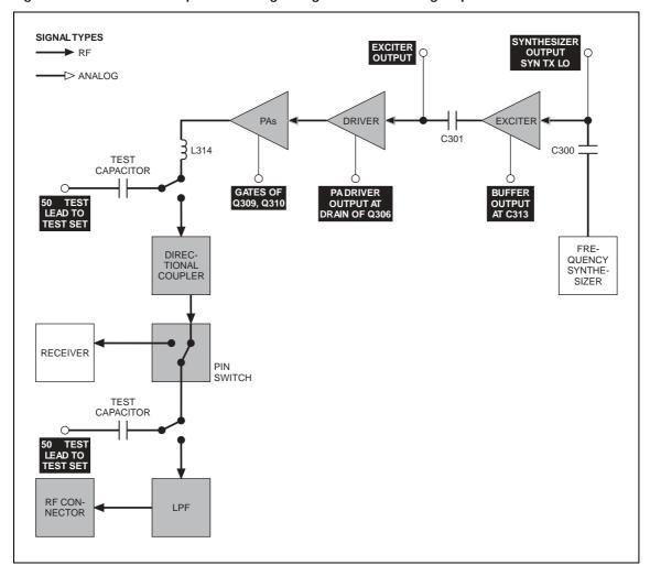
Task 25 — Output of Frequency Synthesizer The first point to check in the initial RF signal path is the output SYN TX LO from the frequency synthesizer. This signal is input to the exciter at C300.
