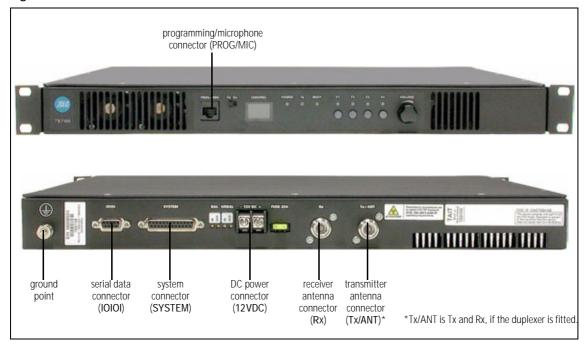
**DC Power** Connector (12V DC) The base station is designed to accept a nominal 13.8V DC, with negative ground.
