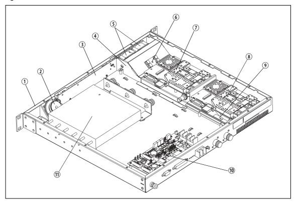
All modules and boards are mounted from above into the 1U tray ①. The modules are secured by screws or clips into standoffs on the tray chassis, and are easily removed for replacement.
