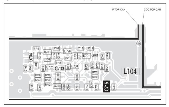
Figure 10.3 Components of the interface circuitry (top side at the corner)
