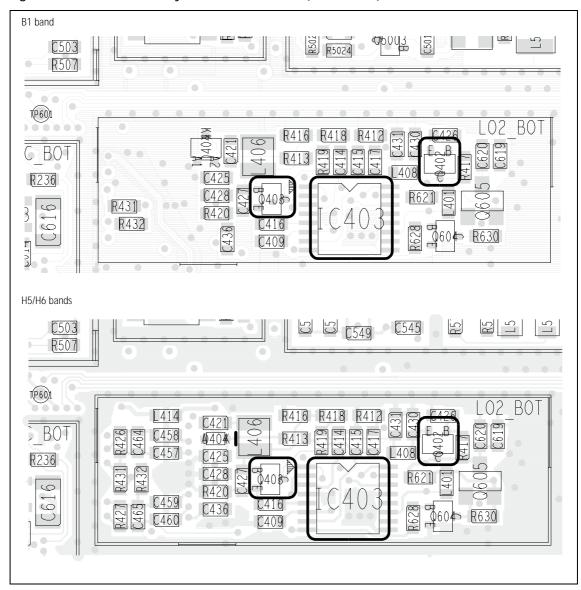
Figure 12.3 Receiver circuitry under the FE TOP can (top side)
