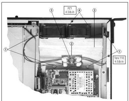
Figure 7.8 Replacing the fans
