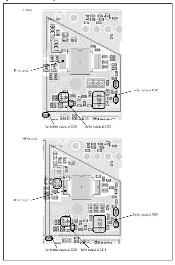
Table 13.8 RF voltages along the initial RF signal path of the VHF radio (B1 band)
