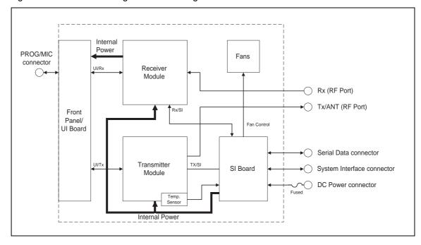
Figure 3.1 Base station high-level block diagram
