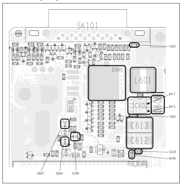
Figure 9.2 Important components of the power-supply circuitry (top side), including 9V regulator IC601
