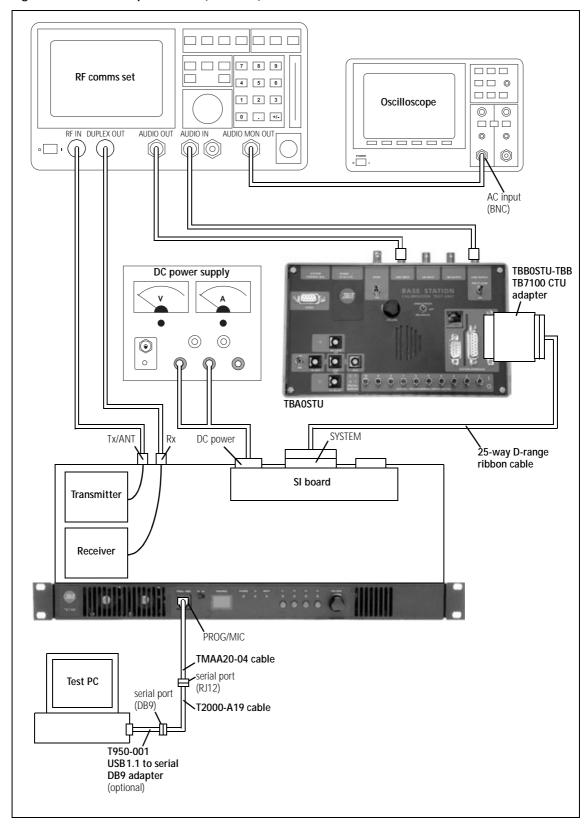
Alternative Test Setup with TOPA-SV-024 Test Unit and TMAC20-0T Control Head An alternative test setup using the TOPA-SV-024 test unit and cables of the TMAA21-00 kit and a TMAC20-0T control head used for testing the transmitter and receiver modules is shown in Figure 6.3.
