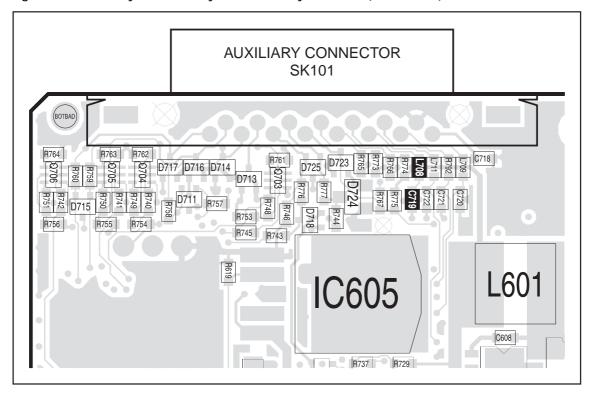
Task 9 — Check LPF and Buffer Amplifier If there is no test signal at the internal-options connector, then either CODEC 1 is faulty or there is a fault in the LPF or buffer amplifier.
