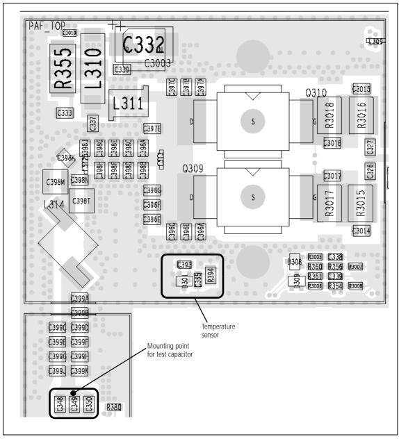
PAF 309 C330 0310 R352  $^{\circ}$ C337 C397E  $\alpha$ C397Q C334 £3987 0309 **-1313**-C331 C399A C399B C396G G C399C C399D  $\infty$ R349 C396F 4 **E399** C399F C396E C3990 C399H 23990 C399I H3005 C338 C399L R360 R358 R3007 C399N C399M R361 C339 R3006 R354 R3008 C399P DIRC TOPESSEN Temperature C3995 C399T sensor C399U C399V C399W C399X . Mounting point **C399 C399** Z for test capacitor
