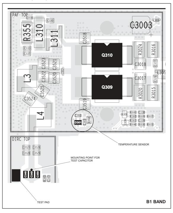
PAF **TOP** C332 L303 310 C3003 1323 C330 C333 R351 Q310 C334 C3520A C327 308 HILL C3521B L307 C3519 C331 Q309 R348 R3005 C338 ¢3522k ¢3522l R360 R356 R3007 R361 C339 R3006 R354 R3008 DIRC TOP 3522 ¢3522\$ ¢3522T TEMPERATURE SENSOR ¢3522µ¢3522V MOUNTING POINT FOR TEST CAPACITOR C348 C349
