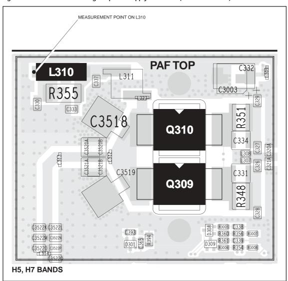
Figure 14.3 Point for measuring the power supply to the PAs (H5 and H7 bands)
