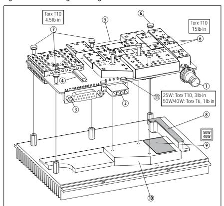
Figure 7.5 Removing and fitting the transmitter board
